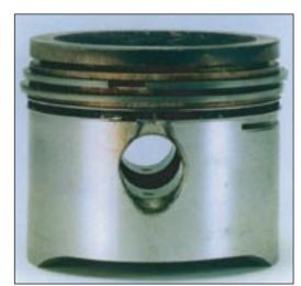
HOLE IN PISTON CROWN. CROWN EDGE BURNING.
