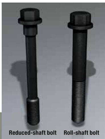
▲ Advantage of stretch bolt: As opposed to a rolled shank bolt, it can be tightened beyond its elastic limit (yield point) into the plastic region – a guarantee for high and uniform bolt clamping forces.
