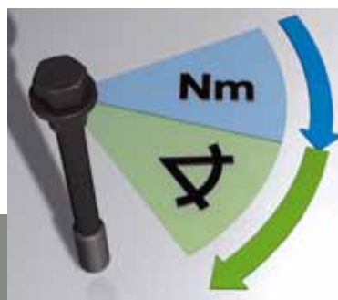
▲ Torque-angle method using pretorque and tightening angle.
